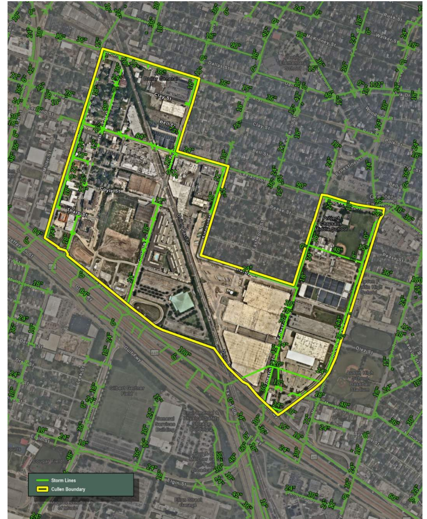
Existing Storm Sewer lines
